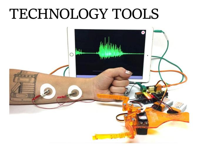
Students used a prefabricated EMGcontrolled gripper throughout the unit. mage credit: Backvard Brains
